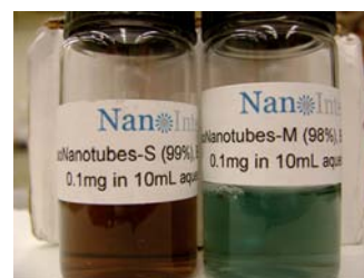
Figure 1. Separated SWNT solutions. (left) S-SWNTs; (right) M-SWNTs.
